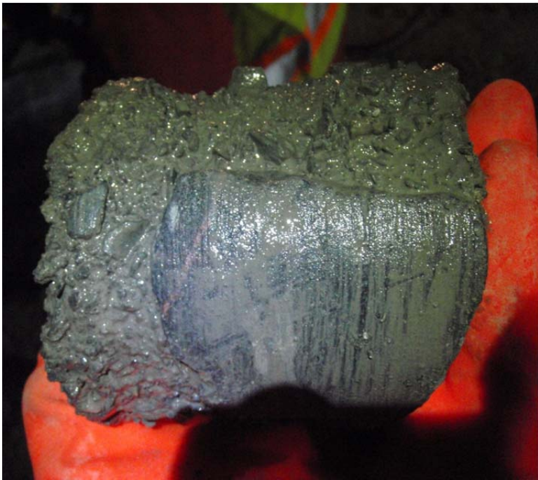
Photo 10: A large piece of rock was hit when coring the lift placed 2012/01/22 near station 1+20 downstream side. A second core was taken a few feet from the first, as the first core was stopped short and of very poor quality (due to drilling). Core HB12-ND-CORE-DC7-20120123 was taken immediately adjacent to this location.
