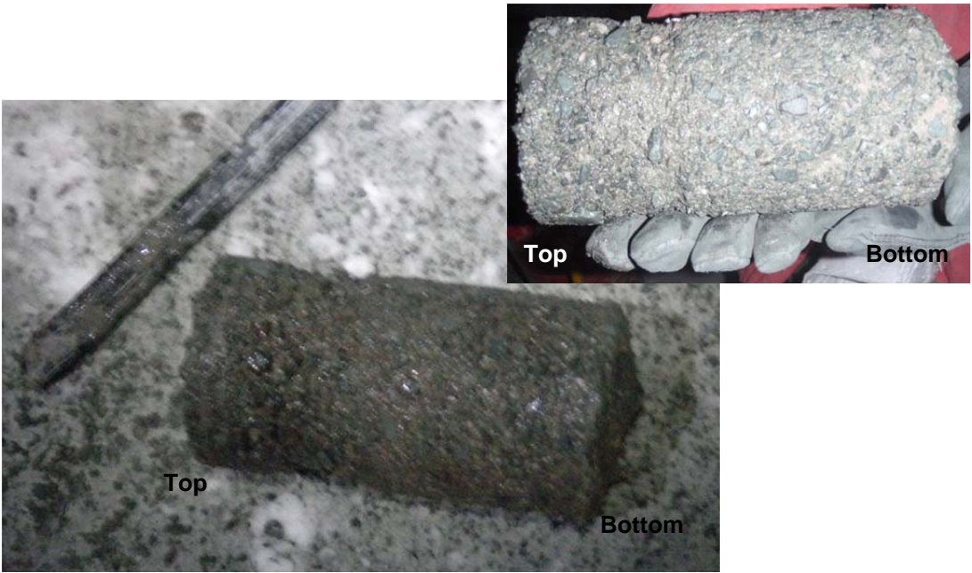
Photo 9 and 10: HB12-ND-CORE-DC6-20120123 collected from Sta. 0+95 center of key trench. Thinning near top of this core is due primarily to drill chatter.
