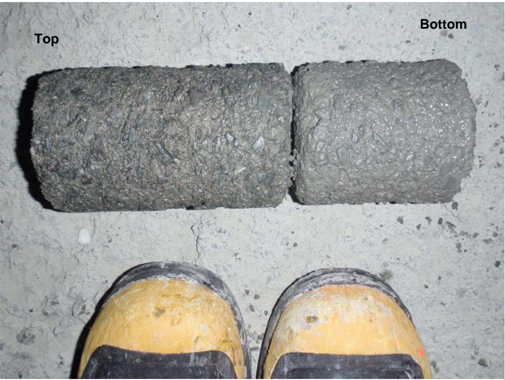
Photo 11 Drilled core HB12-ND-CORE-DC7-20120123 taken at Sta. 1+20 downstream. Note that this core separated (spun off) at the joint between lifts.
